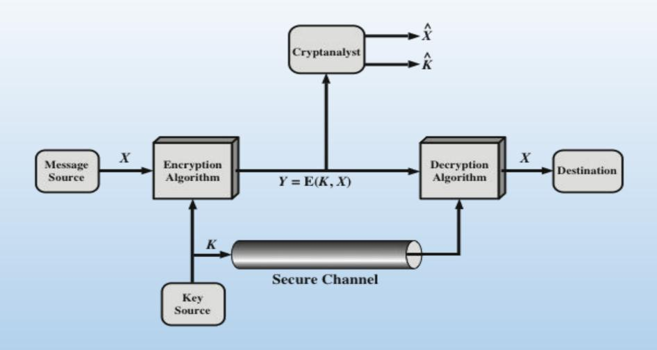
Figure 3.2 Model of Symmetric Cryptosystem
